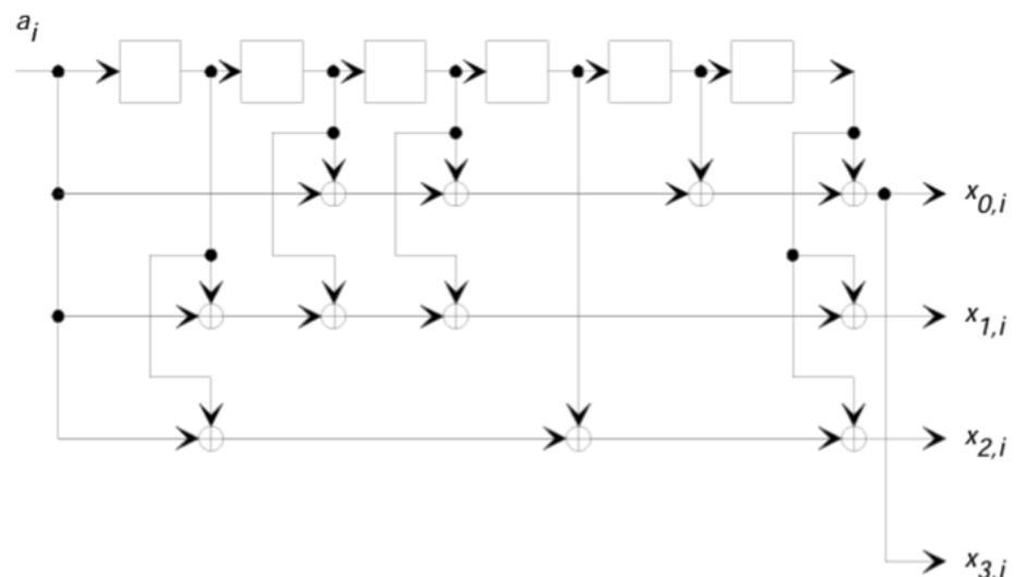
Figure 86: Convolutional encoder
